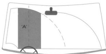
Repaired windscreens are judged on whether the repair interferes with vision. An ‘invisible’ or barely detectable repair, finished flush with the surrounding glass, does not count as damage.
