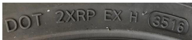
The first two digits of the code represent the week of manufacture of the tyre and the second two digits represent the year of manufacture. In the example above, the tyre was manufactured in week 35 of 2016.
